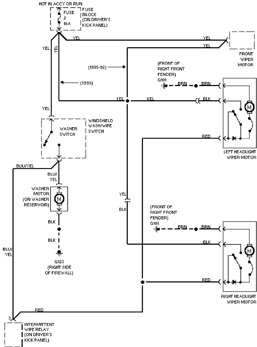
**SYSTEM WIRING DIAGRAMS**
