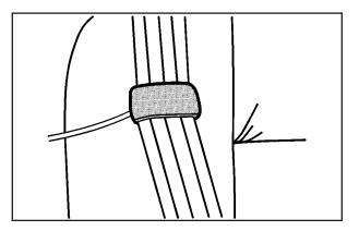
3. Be sure that the belt is not twisted and it lies flat. The elastic cord must be under the belt with the guide on top.
