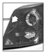
The headlamp washers are located on the inboard side of the headlamp lenses.
