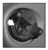
The key cannot be removed from the ignition of manual transmission vehicle unless the key release button is used.
