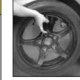
10. Place the compact spare tire on the wheel-mounting surface.
