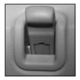
From the inside, use the manual lock levers located on the door panels near the windows.
