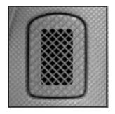
There is also an interior temperature sensor located to the right of the steering wheel on the instrument panel.
