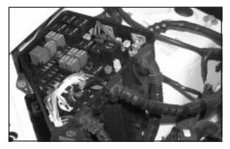
The underhood fuse block is located in the engine compartment on the passenger's side of the vehicle. See *Engine Compartment Overview on page 5-12* for more information on location.
