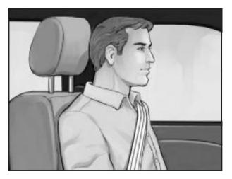
Adjust your head restraint so that the top of the restraint is closest to the top of your head. This position reduces the chance of a neck injury in a crash. The front seat head restraints move up and down. Press the button located at the bottom of the head restraint to raise or lower the head restraint. The head restraints tilt forward and rearward, also.
