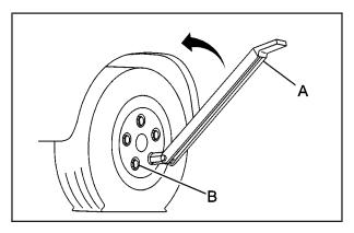
Place the wheel wrench (A) securely over the wheel nut (B). Turn the wheel wrench counterclockwise to loosen all the wheel nuts. Don't remove them yet.
