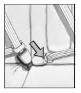
Insert a tool with a small tip into the slot as shown to unlatch the seatbelt buckle. Then move the belt to the side so it is not in your way.
