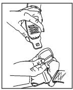
2. Reconnect the center safety belt latch plate to the buckle as shown.
