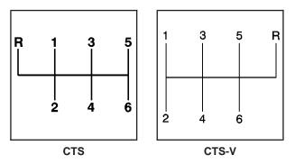
This is the shift pattern for the six-speed manual transmission.
