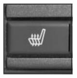
If your vehicle is equipped with heated front seats, the buttons are located on the climate control panel. There is one button for the driver and one for the front passenger. Each button has three settings, LO, HI and off. The active setting appears on the climate control panel display. The LO setting warms the seatback and cushion until the seat approximates normal body temperature. The HI setting has a slightly higher temperature.
