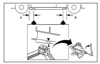
2. Find the jacking location using the diagram above and corresponding hoisting notches located in the plastic molding. The notches in the plastic molding are marked with a triangle shape to help you find them.
