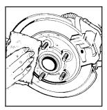
9. Remove any rust or dirt from the wheel bolts, mounting surfaces and spare wheel.
