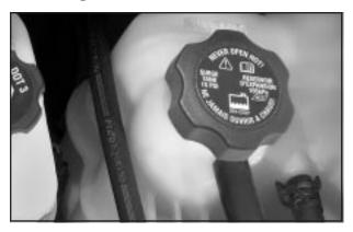
The coolant surge tank and pressure cap are located on the driver's side of the vehicle, toward the rear of the engine compartment. See *Engine Compartment Overview on page 5-12* for more information on location.
