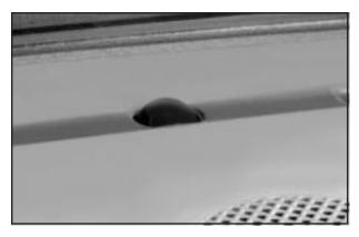
There is a solar sensor located on the instrument panel, near the windshield.
