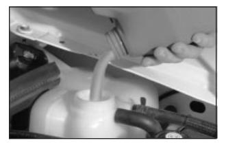
3. Fill the coolant surge tank with the proper mixture, to slightly above the FULL COLD/FROID line on the side of the coolant surge tank.
