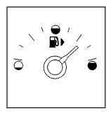
The fuel gage shows approximately how much fuel is in the tank. It works only when the ignition is in ON. If the fuel supply gets low, the Fuel Level Low message will appear on the DIC and a single chime will sound. See *DIC Warnings and Messages on page 3-65* for more information.
