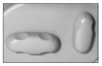
If your vehicle is equipped with power front seats, the controls are located on the outboard sides of the front seat cushions.
