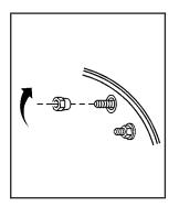
11. Put the wheel nuts back on with the rounded end of the nuts toward the wheel. Tighten each wheel nut by turning it clockwise with your hand until the wheel is held against the hub.
