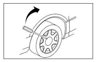
If your vehicle has wheel covers, use the flat end of the wheel wrench to remove the covers. Turn the wheel wrench clockwise to gently pry off the wheel cover.
