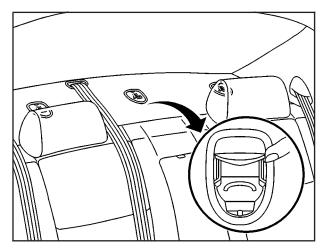
The top strap anchors are located on the filler panel behind the rear seat head restraints. In order to access the anchors, you will have to open the covers. Do not secure a child restraint with a top strap in the right front passenger's position if a national or local law requires that the top strap be anchored, or if the instructions that come with the child restraint say that the top strap must be anchored. There is no place to anchor the top strap in this position.
