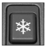
The winter driving mode button is located on the center console near the transmission shift lever.
