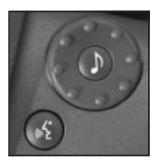
Some audio functions can be adjusted at the steering wheel. They include the following: **Volume:** Turn this knob to increase or to decrease the volume.
