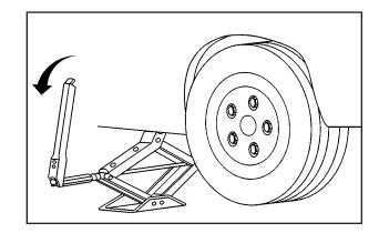
12. Lower the vehicle by turning the wheel wrench counterclockwise. Lower the jack completely.
