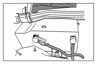
Open the hoods and locate the positive (+) and negative (-) terminal locations of the other vehicle, as well as the positive (+) terminal location on your vehicle's battery. See *Engine Compartment Overview on page 5-12* for more information on the location of the battery.
