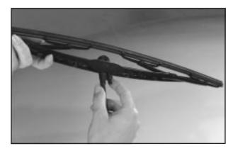
Lift the wiper blade assembly up so it is in a T-shaped position. You should be able to see a tab.
