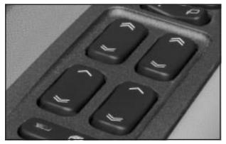
The power window switches are located on the armrest near each window. Press the up or down arrows on the switches to raise or lower the windows.
