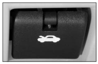
1. Pull the hood release lever inside the vehicle. It is located on the lower left side of the instrument panel.
