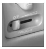
This control is located below the exterior lamps control knob. It automatically turns the lamps on and off by sensing how dark it is outside. To operate the Twilight Sentinel, leave the exterior lamps control knob off and move the TWILIGHT lever to any position but OFF.
