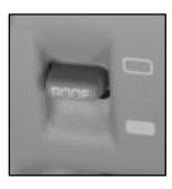
Press and hold the ROOF switch rearward to the first position to open the glass panel and sunshade. The sunshade can also be opened or closed by hand. To close the glass panel, press and hold the ROOF switch forward.
