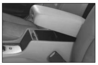
The center console comes with a storage tray, a storage compartment for CDs or tapes, a dual cupholder that unfolds, a coinholder, an optional phone and an armrest. The cupholder can be opened by pressing on the surface panel located in front of the armrest and unfolding it. Close the lid to secure.
