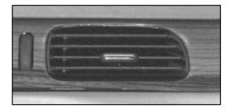
The front outlets are located in the center and at each side of the instrument panel. You can adjust the direction of airflow by moving the center control levers or you can stop the airflow by moving the control dial located on each outlet downward.
