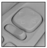
This feature is located on the driver's door armrest. Move the L/R select switch located under the power mirror control to choose the left or right mirror.
