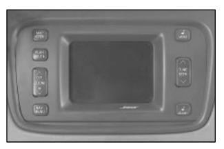
This display screen is located in the center of the instrument panel. There are eight "hard" buttons and a touch sensitive screen.
