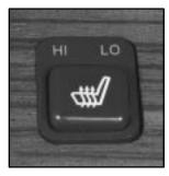
The front seat controls are located in the center console. The rear seat controls are located on the rear door. (Note that only the outboard positions in the rear seats are heated.)
