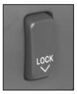
The power door lock switch is located on each front door. Press the top of the switch to unlock all of the doors at once. Press the down arrow (LOCK V) to lock the doors.
