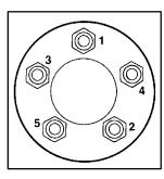
12. Tighten the wheel nuts firmly in a crisscross sequence as shown.
