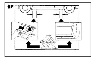
2. Find the jacking location from the diagrams above and corresponding cutouts in the plastic molding.
