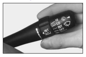
You can control the windshield wipers by moving the lever with the wiper symbol on it. This lever is located on the right side of your steering column. For information on wiper-activated headlamp operation, refer to "Wiper-Activated Headlamps" in the Index.
