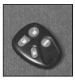
With this feature, you can lock and unlock the doors, unlock the trunk, open the fuel door and turn on your vehicle's interior lamps from about 3 feet (1 m) up to 30 feet (9 m) away using the RKE transmitter supplied with your vehicle.
