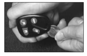
1. Use a coin (or a similar object) to pry open the transmitter.
