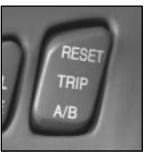
By pressing the bottom of this button, you can tell how many miles you have traveled on either your Trip A or Trip B odometer since you last set the odometer back to zero. Press the RESET part of the button until zeros appear to reset the odometers.
