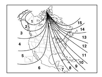
3. Press COMPASS on the bottom of the mirror until the new zone number appears in the display. After you stop pressing the button, the display will show a "C" and will need recalibration.
