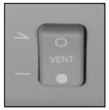
To vent the sunroof, press and hold the upper part of the VENT switch. The sunshade must be opened by hand. To close, press and hold the lower part of the VENT switch.
