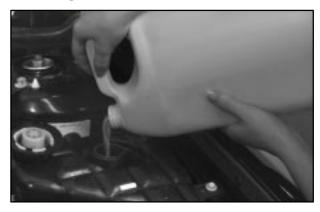
The engine coolant surge tank is located on the driver's side of the engine.
