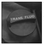
The transaxle fluid cap is located next to the radiator hose and below the air cleaner assembly on the driver's side of the engine.
