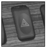
The hazard warning button is located in the center of the instrument panel, between the two air vents. Press the button in to make the front and rear turn signal lamps flash on and off.
