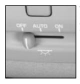
The interior lamps control, located in the overhead console, has three positions: OFF, AUTO and ON.
