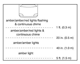
A chime will sound the first time an object is detected, if the object is between 20 inches (0.5 m) and 5 feet (1.5 m) away.
