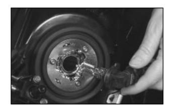
6. Remove the headlamp bulb socket.
