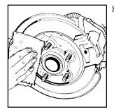
8. Remove any rust or dirt from the wheel bolts, mounting surfaces and spare wheel.
