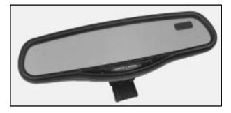
By pressing the MIRROR side of the button located at the bottom of the mirror, the mirror automatically changes to reduce glare from headlamps behind you. The mirror also includes an eight-point compass display in the upper right corner of the mirror face. When on, the compass automatically calibrates as the vehicle is driven.
