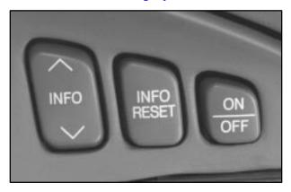
**INFO:** Pressing this button up or down will display the OUTSIDE TEMP, MILES RANGE, MPG AVG, MPG INST, GAL FUEL USED, AVG MPH, TIMER, BATTERY VOLTS OK, ENGINE OIL LIFE, TRANS FLUID LIFE, PHONE (If Equipped) and FEATURE PROGRAMMING.
