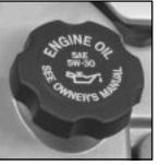
The engine oil fill cap is located behind the radiator on the passenger's side of the engine. Turn the cap counterclockwise to remove it.
