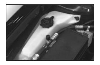
The windshield washer fluid reservoir is located next to the fuse relay center on the passenger's side of the engine.
