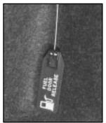
An alternate fuel door release is located inside of the trunk on the driver's side. Pull it to release the fuel door.
