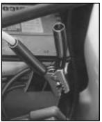
Now connect the black negative (-) cable to the good battery's negative (-) terminal. Don't let the other end of the negative (-) cable touch anything until the next step. The other end of the negative (-) cable *doesn't* go to the dead battery. It goes to a heavy, unpainted metal engine part (on your vehicle, you may use the windshield washer bottle stud as shown). Don't allow the red and black handles on the jumper cable to touch each other.
