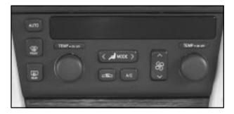
Your vehicle is equipped with a dual-zone electronic climate control system. This system can automatically adjust and control temperature, fan speed, air delivery mode, air conditioning operation and air intake. You can use the AUTO (automatic) setting or override the automatic operation by manually altering the controls. If your vehicle is equipped with the Climate Control Personalization feature, you will be able to program
