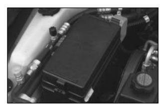
The front Bussed Electrical Center (BEC) is located in the front of the engine compartment between the windshield washer fluid reservoir and the power steering fluid reservoir (on the passenger's side). Lift the cover to gain access.
