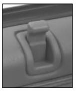
The manual lock is located on the top of the door panel near the window. Push the manual lock lever down to lock the door from the inside. To unlock the door, raise the lock lever.
