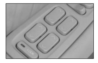
The power window controls are located on the armrest near each window. Press the up or down arrows on the controls to raise or lower the windows.
