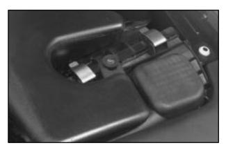
The air cleaner is located next to the coolant surge tank on the driver's side of the engine. Be sure the engine has cooled before following these steps to replace the air cleaner filter:
