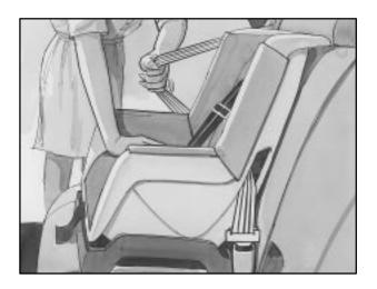
4. To tighten the belt, pull up on the shoulder belt while you push down on the child restraint. If you're using a forward-facing child restraint, you may find it helpful to use your knee to push down on the child restraint as you tighten the belt.
