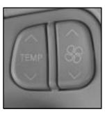
Some heating and cooling controls can be adjusted at the steering wheel. Other touch controls operate some audio controls. See "Audio Steering Wheel Controls" in the Index.
