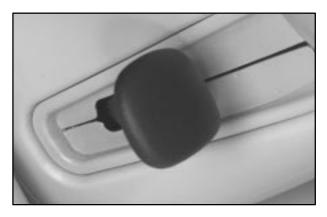
The tilt wheel control is located on the outboard side of the steering column. Tilt steering allows you to adjust the steering wheel before you drive. Raising the steering wheel to the highest level gives your legs more room when you enter and exit the vehicle.
