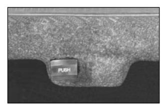
The rear seat pass-through release button is located in the trunk. To release the pass-through door, press the PUSH button located in the center of the trunk panel.
