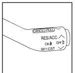
The cruise control lever is located on the lower right side of the steering column.
