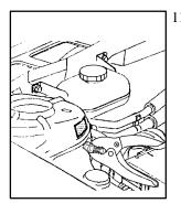
11. Attach the cable at least 18 inches (46 cm) away from the dead battery, but not near engine parts that move.
