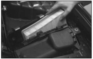
5. Take out the air cleaner filter and remove any loose debris that may be found lying in the air cleaner base.
