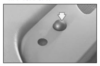
The sensor monitors the sun's solar radiation and is located near the end of the instrument panel near the windshield.
