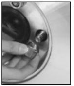
10. Replace the wheel nuts with the rounded end of the nuts toward the wheel. Tighten each nut by hand until the wheel is held against the hub.
