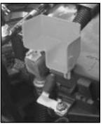
6. Start by lifting and moving the red positive (+) remote terminal cover away from the relay center.
