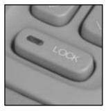
Press the LOCK button down to disable the rear passenger's window controls. A light on the button will display to indicate that the rear window controls are disabled.
