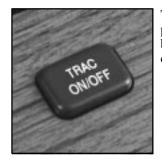
To turn the system off, press the TRAC ON/OFF button located on the center console.
