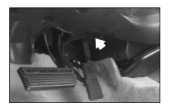
The filter is located inside the air control module, with an access panel under the instrument panel near the accelerator pedal. The filter should be replaced as part of routine scheduled maintenance. See the Maintenance Schedule booklet for replacement intervals. See your dealer for details on changing the filter.
