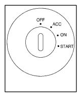
**OFF:** This position lets you turn off the engine and remove the key. This position also locks the steering wheel and transaxle.
