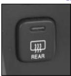
The grid lines you see on the rear window warm the glass. Press this button to turn on the rear defogger. With it, the rear window and both outside rearview mirrors are heated. The light on the button will come on while the system is activated.
