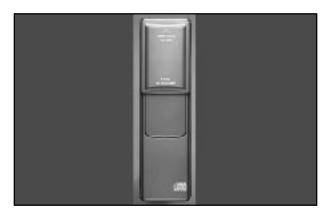
With the compact disc changer, you can play up to six discs continuously. Normal size discs may be played using the slots supplied in the magazine.
