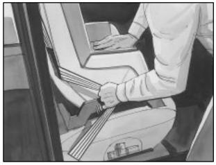
5. Pull the rest of the lap belt all the way out of the retractor to set the lock.
