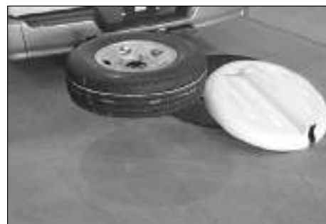
Picture B-P39: Remove catch pin and lower carrier to remove tire.
