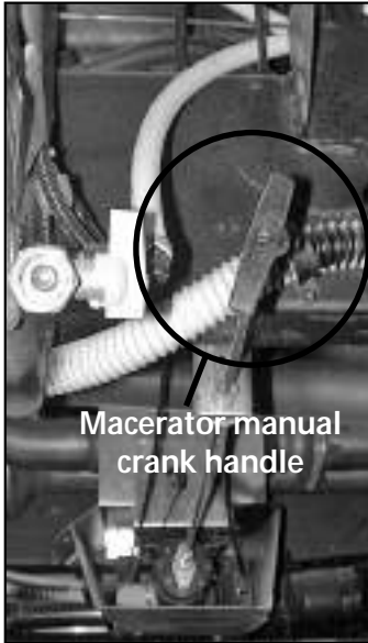
Picture G-P15: Macerator pump located under center of vehicle.
