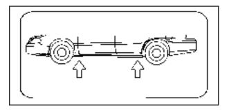
4. To identify the appropriate jacking location, find the triangle about 12 inches (30.5 cm) from the front tire or about 10.5 inches (27 cm) from the rear tire.
