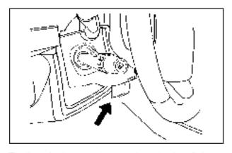
To tilt and telescope the steering wheel, pull down the lever. Then move the steering wheel up or down or backward or forward into a comfortable position. Pull the lever up to lock the steering wheel in place.
