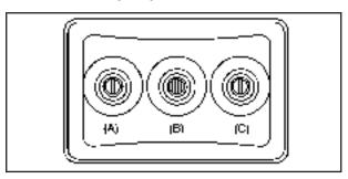
The A/V jacks located on the rear of the floor console, allow audio or video signals to be connected from an auxiliary device such as a camcorder or a video game unit to the RSE system. Adapter connectors or cables may be required to connect the auxiliary device to the A/V jacks. Refer to the manufacturer's instructions for proper usage.
