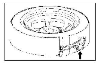
Remove the plastic spare tire heat shield by pulling the rubber latch. Store the plastic spare tire heat shield. See Storing a Flat or Spare Tire and Tools on page 472 for more information.
