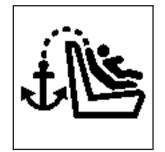
To assist you in locating the top tether anchors, the top tether anchor symbol is located on the trim cover or near the anchor.
