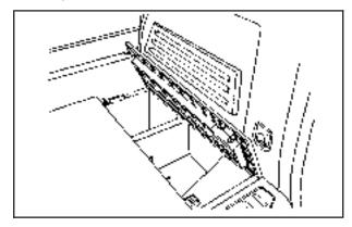
There is an additional storage compartment on each side of the system. To open, unsnap and lift the panel up.
