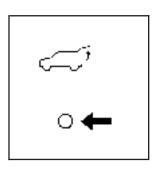
To change the liftgate to manual operation, toggle the switch on the center console to the disable position indicated by a circle.
