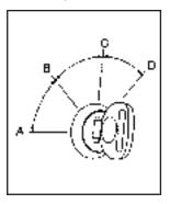
**A (OFF):** This is the only position in which you can remove the key. This position locks the ignition and transmission.
