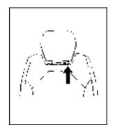
Pull the head restraint up to raise it. To lower the head restraint, press the release button, located on the top of the seatback, while you push the head restraint down.
