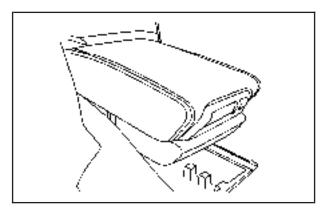
The armrest on the center console can slide forwards and backwards by holding up the lever located on the front of it. To open the armrest storage area, press the button located on the front of the armrest. There is additional storage under the armrest. Move the armrest all the way to the rear position. The tray can be removed for additional storage.
