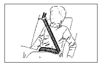
Buckle, position, and release the safety belt as described in Rear Seat Passengers on page 40. Make sure that the shoulder belt crosses the shoulder.
