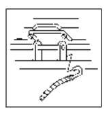
Hook the other end of the cable onto the outside portion of the liftgate hinge (B).
