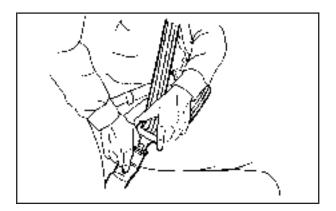
To unlatch the belt, push the button on the buckle. The belt should go back out of the way. When the safety belt is not in use, slide the latch plate up the safety belt webbing. The latch plate should rest on the stitching on the safety belt, near the guide loop on the side wall.
