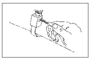
Disconnect the rear safety belt mini-latch, using a key in the slot on the mini-buckle, let the belt retract into the headliner. Stow the mini-latch in the holder located in the headliner.
