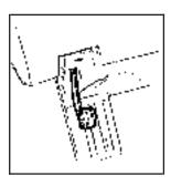
To set the parking brake, push down the parking brake pedal down with your left foot.
