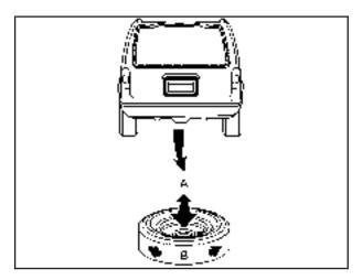
Make sure the tire is stored securely. Push, pull (A), and then try to turn (B) the tire. If the tire moves, use the lug wrench to tighten the cable.
