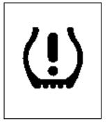
As an added safety feature, your vehicle has been equipped with a tire pressure monitoring system (TPMS) that illuminates a low tire pressure telltale when one or more of your tires is significantly under-inflated.
