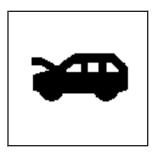
Pull the hood release handle with this symbol on it. It is located under the instrument panel on the driver's side of the vehicle.
