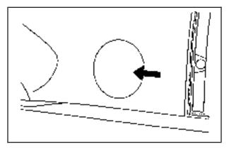
To open the fuel door, push the rearward center edge in and release. The door will pop open.
