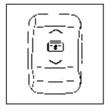
**Vent:** From the closed position, press and hold the front of the driver's side switch to vent the sunroof. Press and hold the rear of the driver's side switch to close the sunroof.
