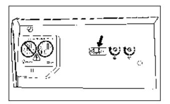
Locate in the garage, the garage door opener receiver (motor-head unit). Locate the "Learn" or "Smart" button. It can usually be found where the hanging antenna wire is attached to the motor-head unit and may be a colored button. Press this button. After you press this button, you will have 30 seconds to complete the following steps.
