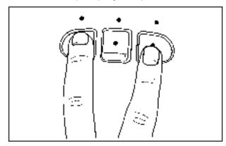
1. From inside the vehicle, press the two outside buttons at the same time for one to two seconds, and immediately release them.
