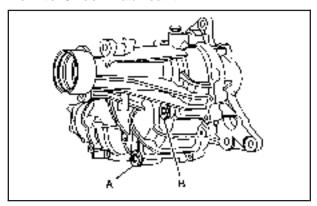
(A) Drain Plug (B) Filler Plug
