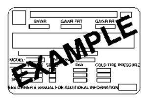
A vehicle specific Certification/Tire label is attached to the rear edge of the driver's door.
