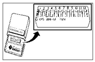
To verify if you have a Fixed Code garage door opener, remove the battery cover on your hand held transmitter supplied by the manufacturer of your garage door opener motor. If you see a row of dip switches similar to the graphic above, you have a Fixed Code garage door opener. If you do not see a row of dip switches, return to the previous section for Programming Universal Home Remote – Rolling Code.
