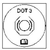
The brake master cylinder reservoir is filled with DOT-3 brake fluid. See Engine Compartment Overview on page 396 for the location of the reservoir.
